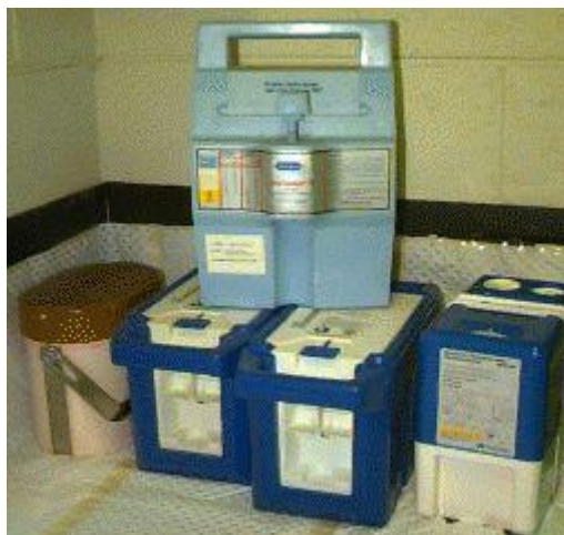
Figure 106 A technetium generator in a hospital (Image by Kieran Maher, Wikimedia Commons)
